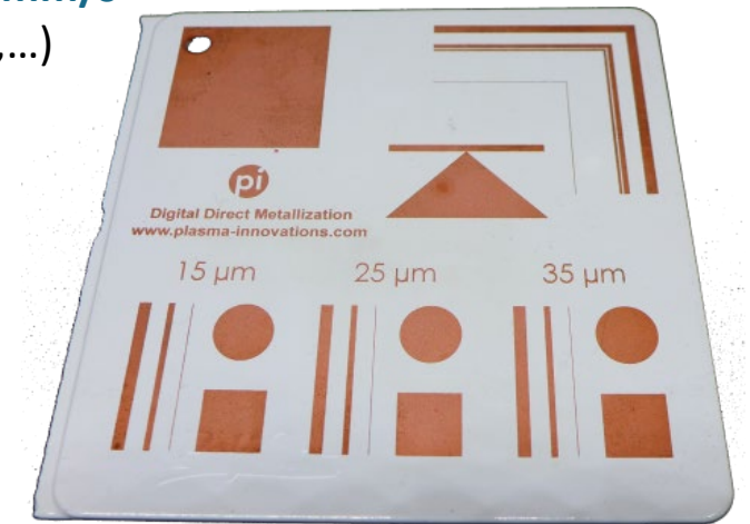
Different Cu-tracks on PA substrate – the shapes were created by locally applying an anti-adhesive varnish
