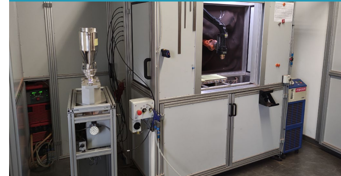
R2R 2D-functionalization setup Roll width of 500 mm
